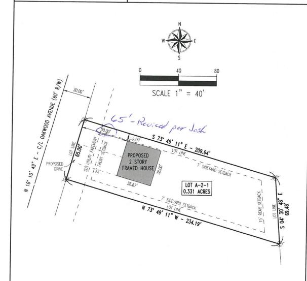
5' OFFSET WOOD HUBS WILL BE PLACED AT EACH CORNER OF OUTSIDE BOX OF PROPOSED HOUSE. THE DISTANCES SHOWN ARE FROM THE BUILDING TO THE LOT LINE. DISTANCES DO NOT GO TO THE EAVES OF THE HOUSE.
